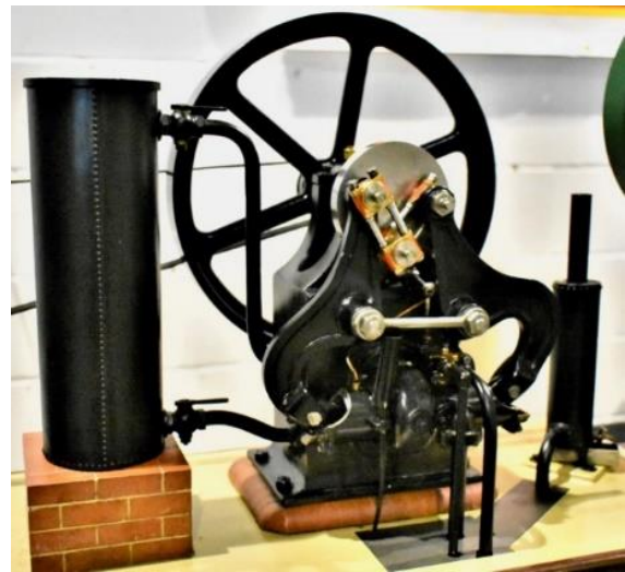
An Atkinson Differential engine in miniature
