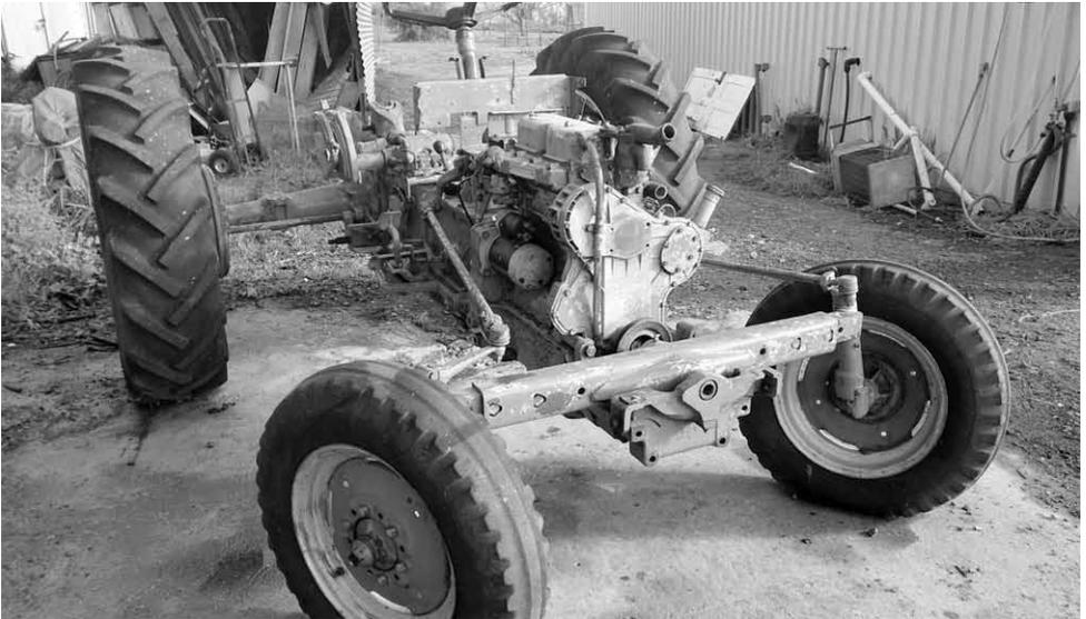
Thomas Elson was called in to fix oil leaks in the front and rear main seals in the engine, fit new trumpet housing gaskets, check the clutch and take care of any other mechanical work.
